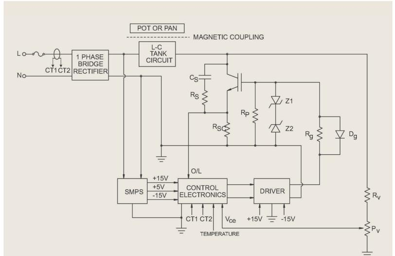
Figure 4: Block diagram of induction cooker
