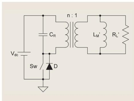
Figure 1: Single switch induction heating circuit
