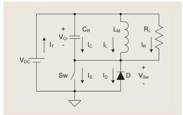
Figure 3: Operating modes of the induction heating circuit
