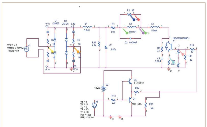
Figure 5: OrCAD schematic of the induction cookert
