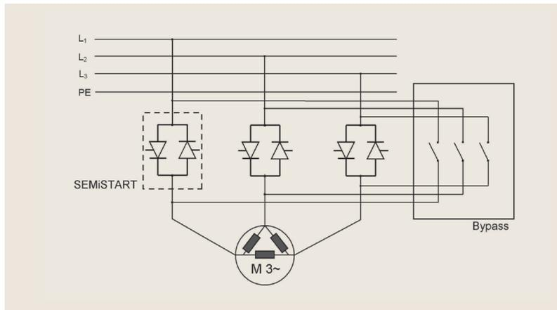
Figure 3: Principle schematic of a soft starter
