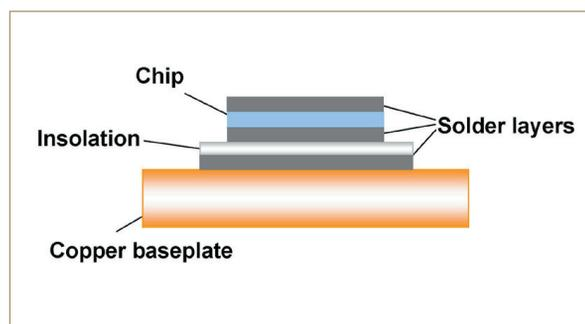
Figure 4: Principle behind the solder contact module
