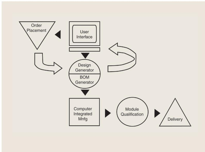
**Figure 2: Custom module design system overview diagram**
