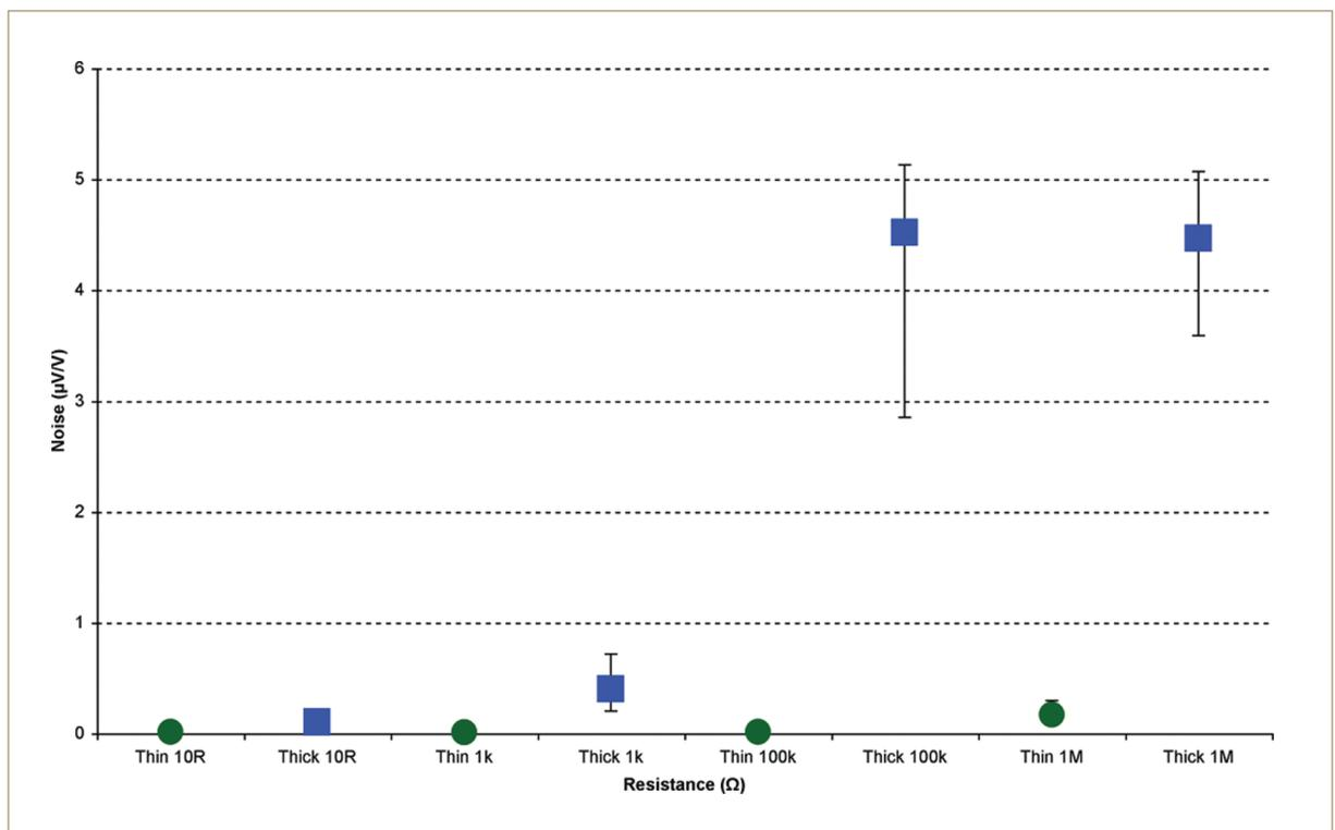
Figure 5: Noise generation of thin and thick-film resistors
