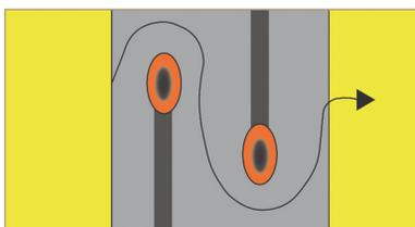
**Figure 1: Laser trimming of the resistor's resistance material eliminates hot spots**
