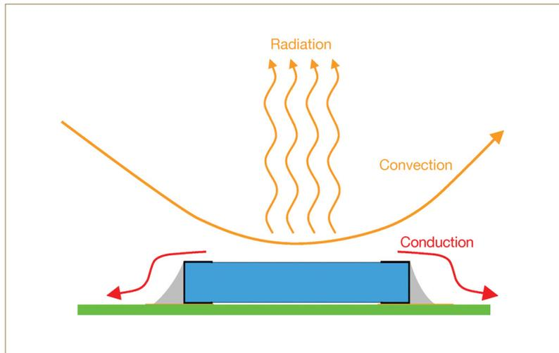
Figure 4: Inverse geometry improves temperature conduction
