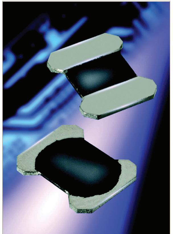
mechanical stress on the resistor. With the change of temperature, the resistor material expands and constricts, which implies a mechanical stress on the solder joint. By reducing temperature
