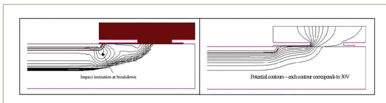
**Figure 4: Forward diode impact ionisation (left) and reverse diode potential contour at a breakdown voltage of 375V**
