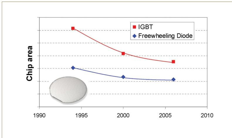
**Figure 2: Development of chip size for IGBT and freewheeling diodes in the last decade. Improvements in the device technology lead to a significant decrease of chip area. This trend however, seems to slow down, due to the fact that it is more and more difficult to manage the heat generated in the power semiconductor devices**
