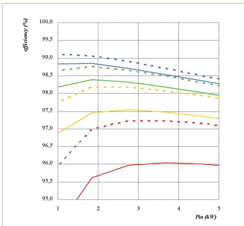
**Figure 5: Efficiency comparison 2x fast 300V FRED versus SiC-diode. The frequency steps are given from 50 to 400kHz in x2 steps**
