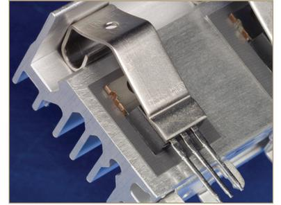
Application of Sil-Pad 1200 for silicone based fiberglass-reinforced thermal interface material solutions that improve performance
