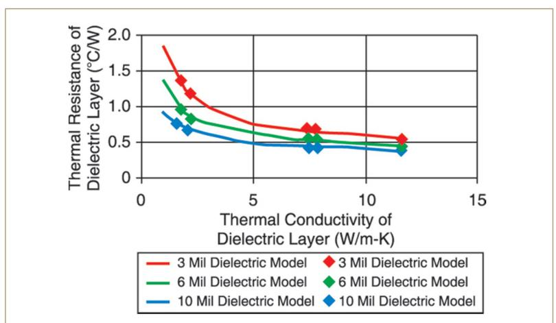
**Figure 2:** Thermal impedance versus thermal conductivity at different thicknesses for the dielectric layer
