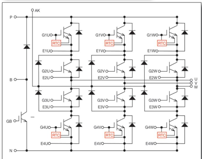
Figure 2: Three-level IGBT module topology including circuitry
