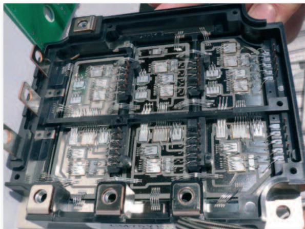
Figure 1: Opened three-level IGBT module
