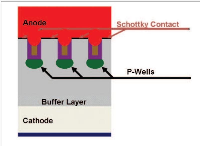
**Figure 3: Internal structure of a Qspeed diode**
