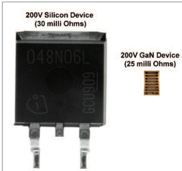
Figure 2: Size comparison between Silicon devices and GaN devices rated at 200V
