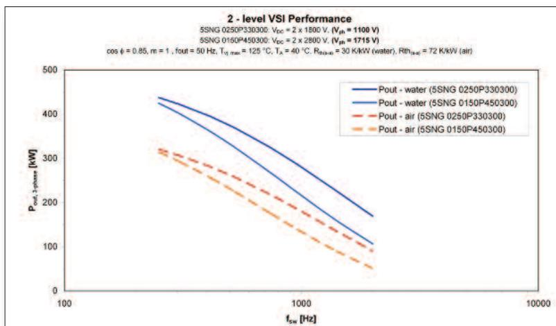
Figure 2: Output power versus switching frequency for a 2-level inverter
