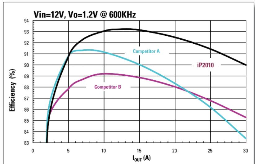
**Figure 6: Measured power conversion efficiency for initial GaNpowiR product (iP2010), a 12V to 1.2V POL converter power stage operating at 600kHz compared to two Silicon based alternatives**
