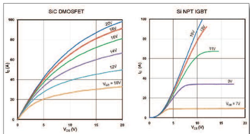
Figure 1: Output characteristics comparison ( $T_j = 150^\circ\text{C}$ )
