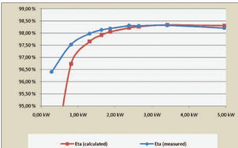
Figure 7: Calculated and measured efficiency of the prototype at  $U_{dc}=800V$
