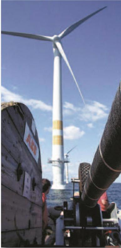
Figure 4: Sea cable for an HVDC Light™ system is laid out for connection of an off-shore wind park to the main land grid
