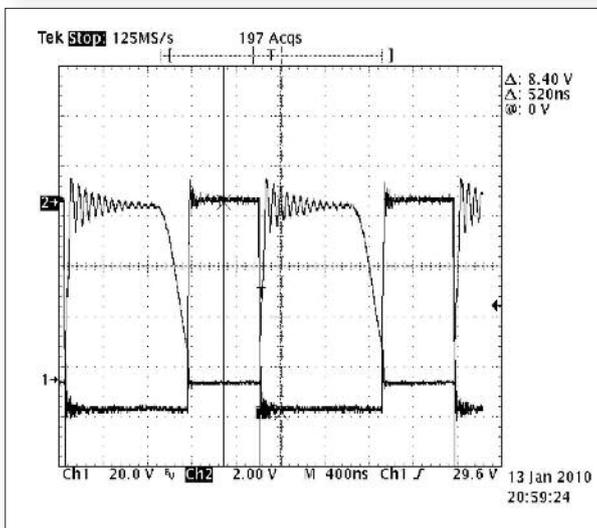
Figure 5: GaN switching waveforms ( $V_{gs}$  and  $V_{ds}$ )
