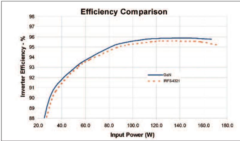
GaN on Si substrate is compatible with established high volume manufacturing facilities and equipment and has the potential to deliver the proper performance/cost benefit.
