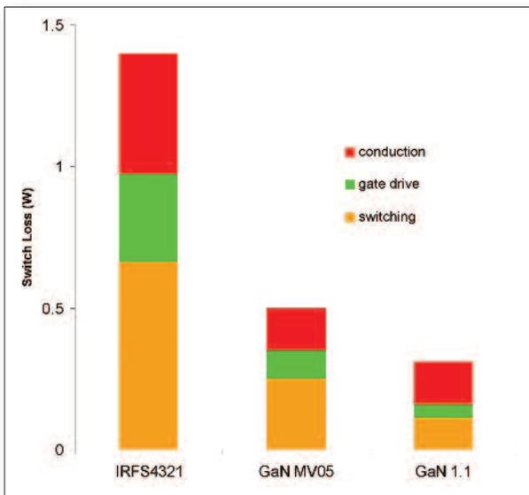
Figure 4: Primary switch power loss breakdown at 170W
