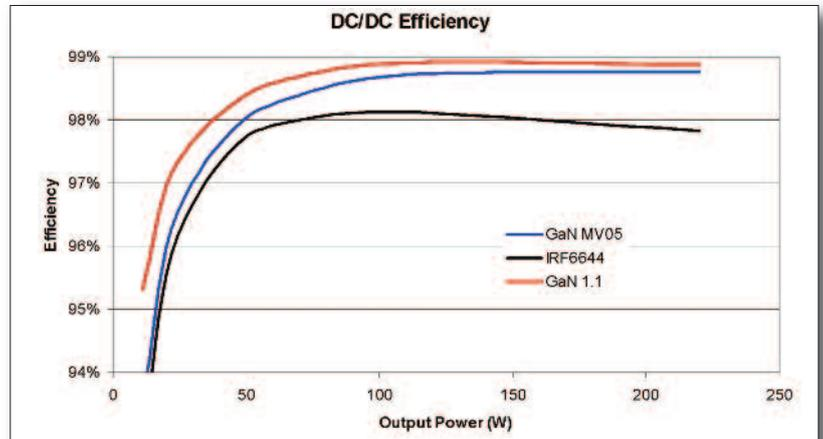
**Figure 9: Buck-boost efficiency at 40Vin**
