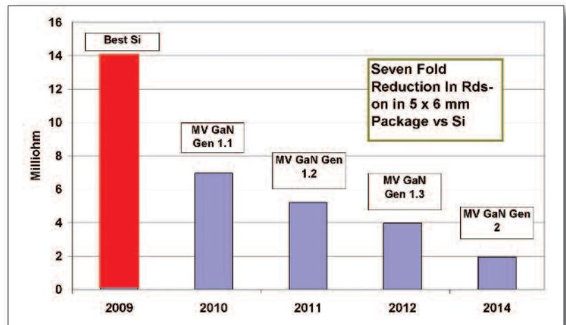
conversion efficiency, all these topologies require the power MOSFETs with the lowest possible specific  $R_{DS(on)} \times Q_C$  FOM. GaN based MOSFETs show great potential in FOM improvement over the coming years (Figure 2).
