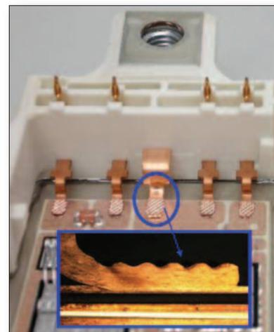
Figure 4: EconoPACK™4 with highly reliable ultrasonic welding for the terminals
