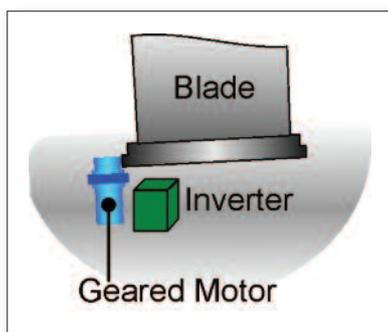
Figure 2: Pitch-Control system for a single blade
