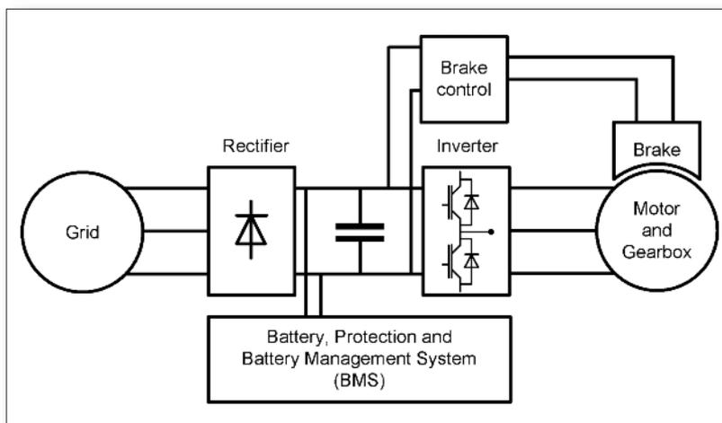
Figure 3: Electric setup of the pitch-control drive
