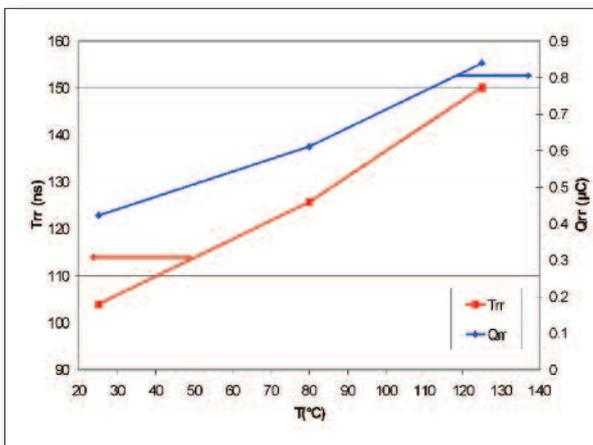
Figure 5: Dependence of  $Q_{rr}$  and  $t_{rr}$  with temperature for the  $310m\Omega$  650V CFD2 device
