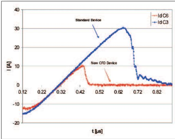
Figure 3: Measured reverse recovery waveforms at  $di/dt=100A/\mu s$ ,  $25^{\circ}C$ ,  $V_r=400V$ . The new CFD device shows very low  $Q_{rr}$ ,  $t_{rr}$  and  $I_{rm}$  when compared to the standard device
