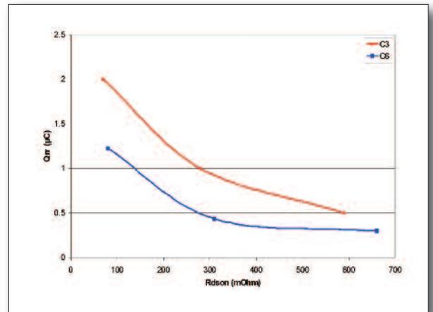
Figure 6: Dependence of  $Q_{rr}$  on  $R_{ds(on)}$ , measured at  $25^{\circ}C$  and for the  $80, 310$  and  $660m\Omega$  650V CFD2 devices in comparison with the former 600V CFD technology
