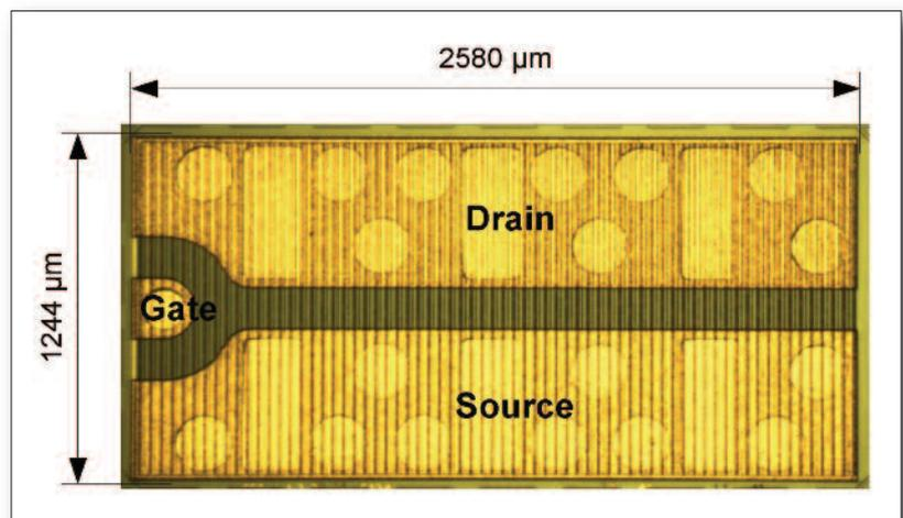
Figure 1: Extremely area efficient Normally-On 600V 180mΩ GaN-HEMT with  $R_{on} \cdot A$  of 570mΩmm<sup>2</sup>
