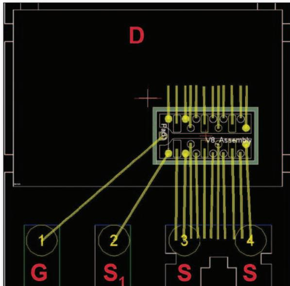
**Figure 3: Normally-on power switch in Infineon's 8x8 ThinPAK**
