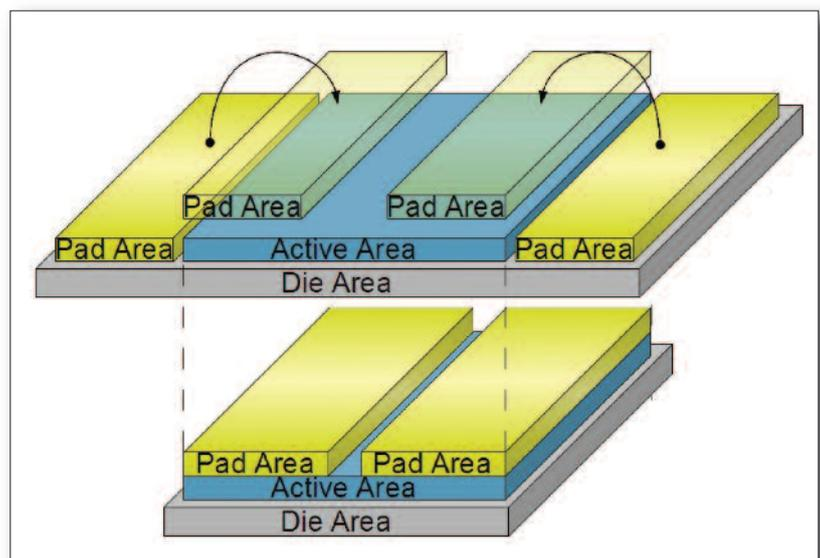
Figure 2: Schematic of MicroGaN's 3D-GaN Technology
