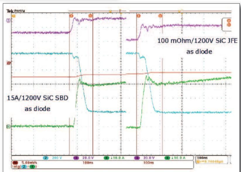
**Figure 2: Comparison of hard commutation of the body diode of a 100mΩ/1200V SiC JFET (right) vs the recovery performance of a 1200V/15A SiC Schottky barrier diode (left) at load current  $I=30A$ ,  $V_{DS}=800V$ ,  $R_g=3\Omega$ ; (Channel 2: Drain voltage, Channel 3: Gate voltage, Channel 4: Current; time base 100ns/div)**
