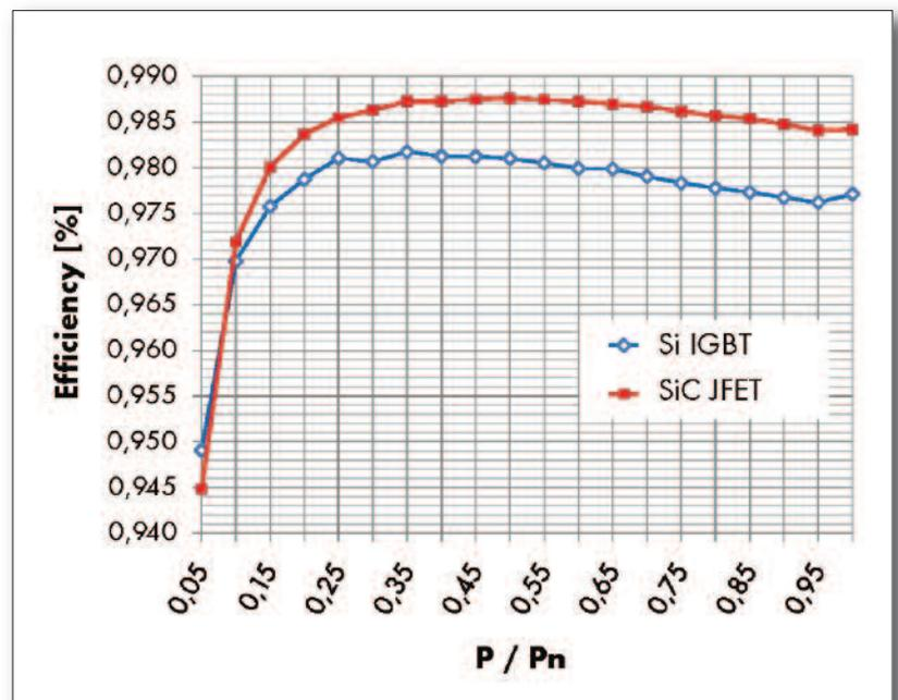
Figure 11: Measured system efficiencies at optimum operation point
