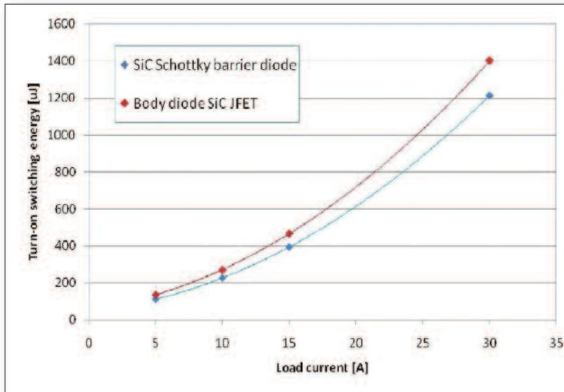
Figure 3: Comparison of turn-on losses of the new 1200V/100mΩ SiC JFET with a 1200V/15A SiC Schottky barrier diode versus the body diode of the SiC JFET as freewheeling diode at  $V_{DS}=800V$ ,  $T_I=75^{\circ}C$ ,  $R_{\theta}=3\Omega$
