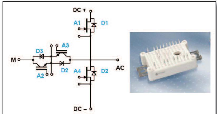
Figure 7: Semiconductor inverter module Easy1b and its PV specific equipment
