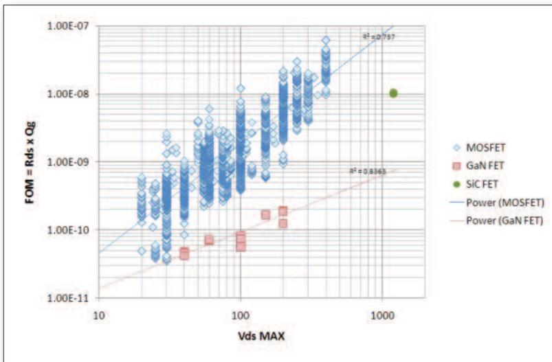
Figure 2: FOM ( $R_{\text{ds}} \times Q_{\text{g}}$ ) for various FET devices currently available on the market. The dots represents different devices, the continuous line is a linear extrapolation for different  $V_{\text{ds}}$ . It is clear that eGaN will be even more competitive for the future generation which will have much higher BV
