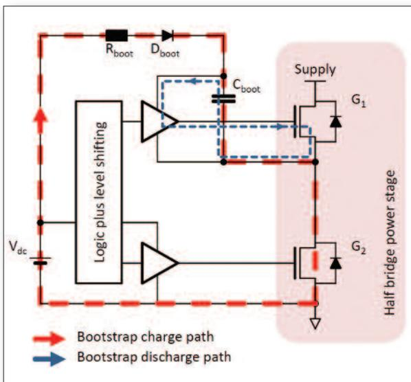
Figure 3: High voltage half bridge and gate driver, shown are high and low-side driver, bootstrap circuit and level shifter
