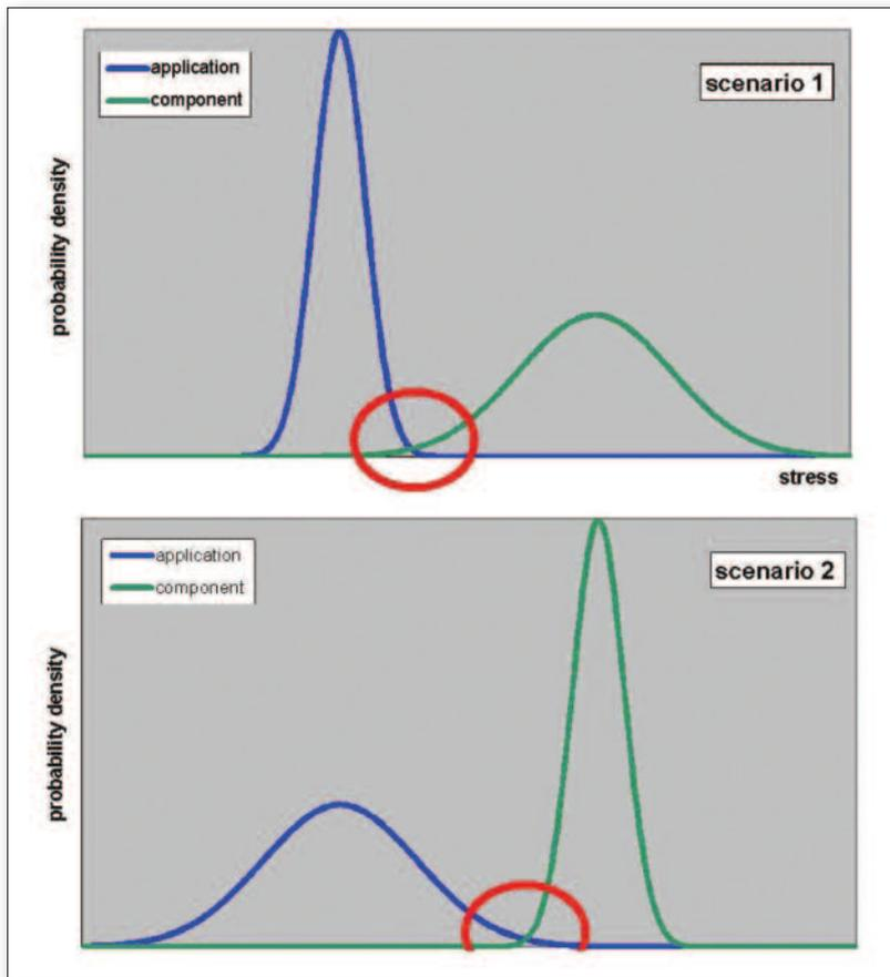
**Figure 3: Comparison of application stress demand and component stress capability: Scenario 1 (top) shows a well-defined application and a component with a large variation of stress capability, while scenario 2 illustrates a well-defined component with a wide distribution of stress for individual instances of the application**
