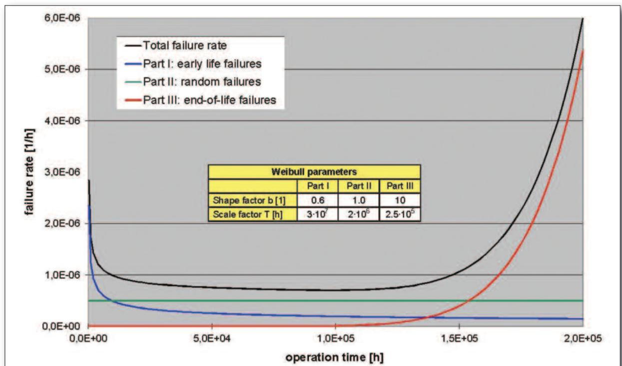
Figure 1: 'Bathtub curve' for a hypothetical power electronic system constructed as the sum of three Weibull distributions representing early life failures (blue), random failures (green) and end-of-life failures (red)
