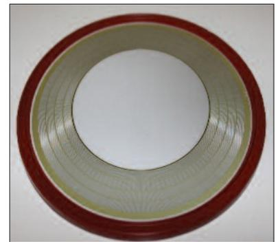
**Figure 9:** Prototype of 150mm 4.5 kV RC-IGCT
