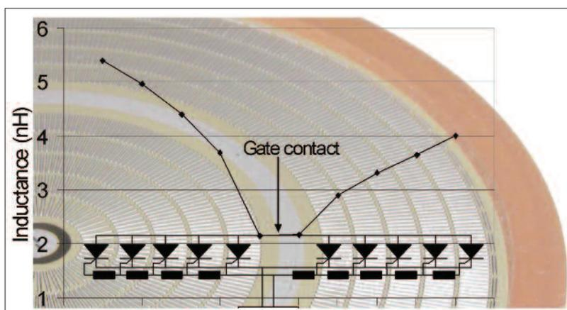
**Figure 2: Inductive situation (simulated values) of the individual segment rings on an IGCT wafer showing how inductances can be distributed over the wafer. The rings far away from the gate contact are more heavily loaded by inductance than the rings in the vicinity. Hence, the gate signal will propagate at some finite speed and disfavor the gate-remote regions**
