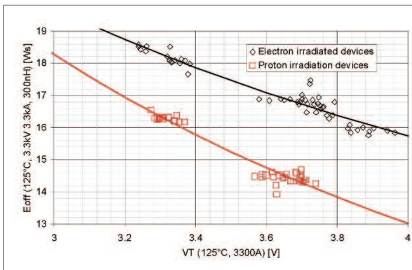
Figure 7: Loss trade-off for the 5.5 kA IGCT switching 3.3 kA at 3.3 kV with a  $T_i$  of 125°C. Additional circuit parameters are listed in the caption of Figure 3
