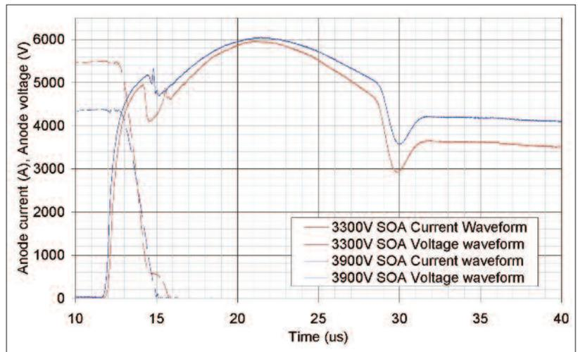
**Figure 4: Current handling capability of the 5.5 kV HPT IGCT. At 3.3 kV DC-link voltage, more than 5.5 kV can be controlled (device testing stopped without destruction). At 3.9 kV, the tests stopped at around 4.4 kA, as the over-voltages involved exceed 6 kV, and hence the specified device capability by more than 500 V**
