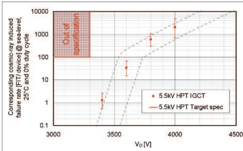
**Figure 8:** Corresponding failure rates due to cosmic rays measured using biased devices in a high-energy proton beam. The specification can be used arbitrarily; however, the 100 FIT level has become the accepted standard where failures due to cosmic rays will become a significant factor in the field
