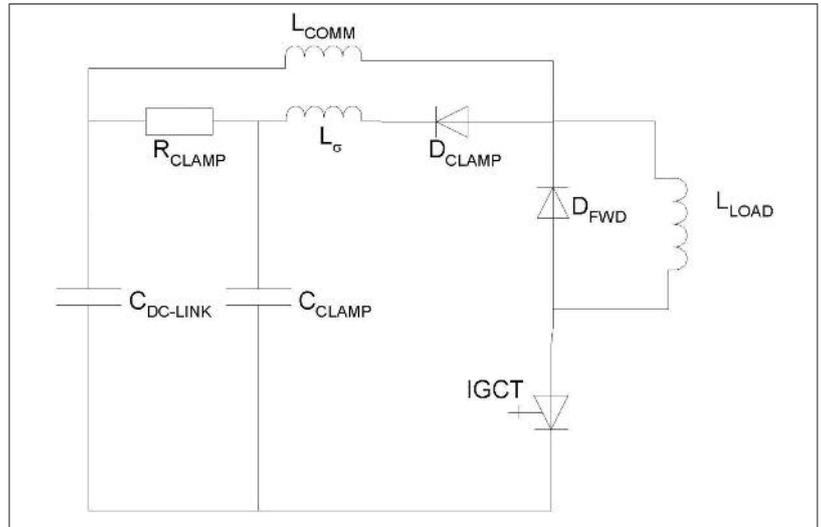
**Figure 3: Circuit used in dynamic testing of the IGCTs (parameters:  $C_{CLAMP} = 8\mu\text{F}$ ,  $L_G = 300\text{nH}$ ,  $R_{CLAMP} = 0.6\ \Omega$ ,  $L_{COMM} = 6\ \mu\text{H}$ )**
