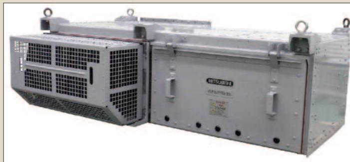
Applying a SiC power module the volume of a railway inverter box is reduced by 42 % and the mass by 37 % compared to a conventional design with Silicon power modules
