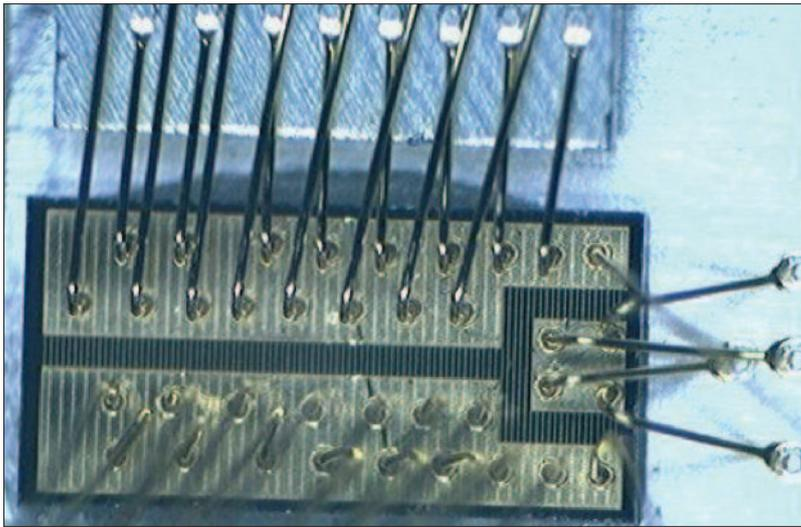
Figure 3: Standard packaging technology compatible pad areas
