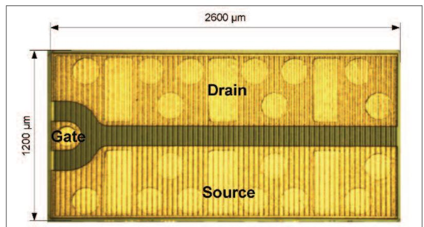
Figure 4: 600 V / 170 mΩ normally-on switch (full device area ~570 mm<sup>2</sup>)
