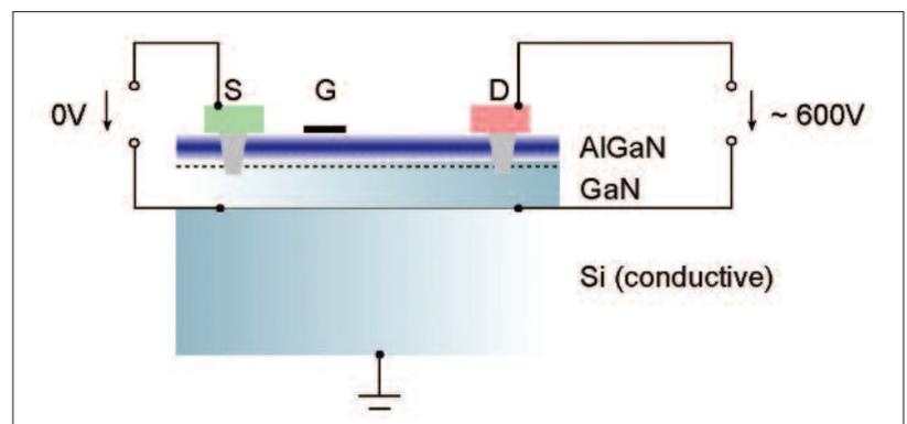
Figure 1: Typical epitaxial structure of GaN-on-Silicon substrates and potential nodes
