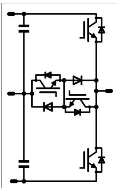
**Figure 4: Single-phase Mixed Neutral Point Converter**
