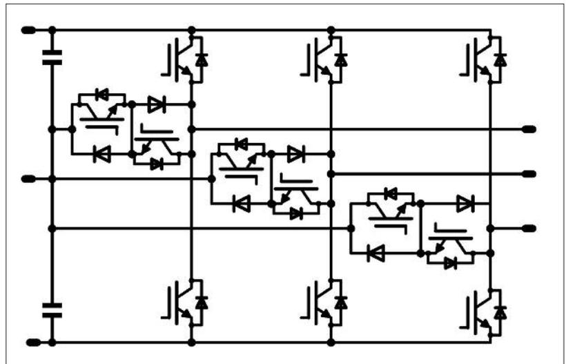
**Figure 5: Integrated three-phase Mixed Neutral Point Converter**
