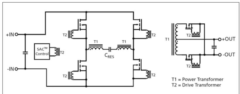
**ABOVE Figure 1: A SAC™ (Sine Amplitude Converter) is a resonant topology that switches its power MOSFETS at fixed frequency at zero-crossing points. The topology reduces power dissipation and high-order harmonics**
