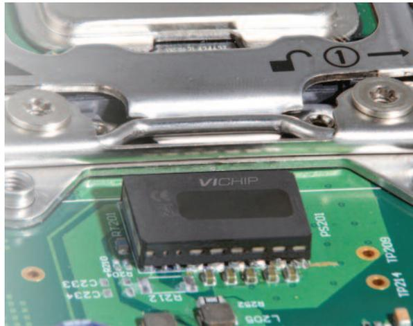
**Figure 5:** A 1323 size VTM current multiplier ChiP supports a tight layout, supplying a processor directly from a 48-V bus with no PoL bulk capacitors
