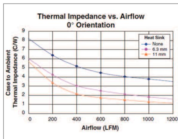
**LEFT Figure 2: Heatsinks reduce case to ambient thermal impedance, shown here as a function of airflow over a representative encapsulated power module**
