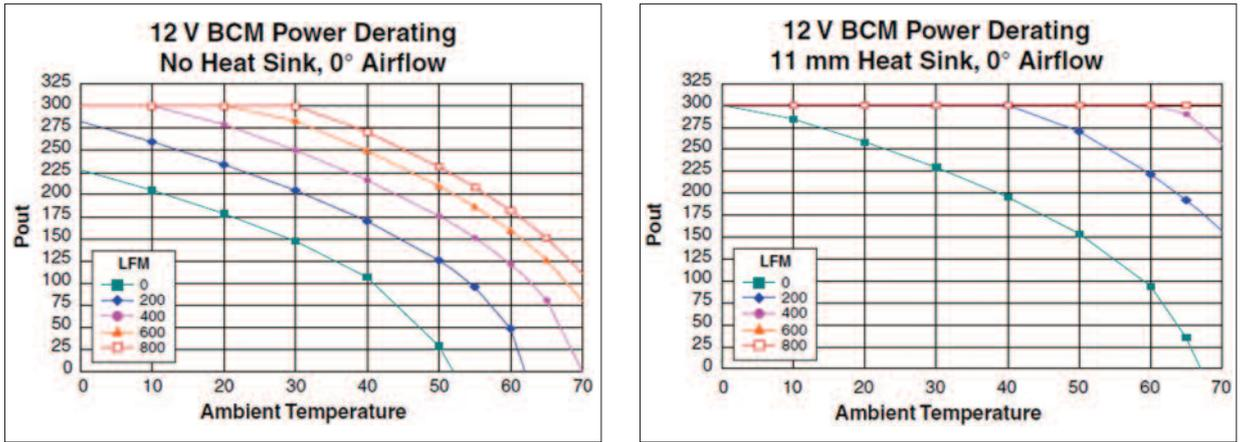
Figure 3: Derating curves, such as these for a Vicor 12-V BCM show the effect of airflow on realizable power capacity in designs with no heat sink (left) and with an 11-mm heat sink (right)
