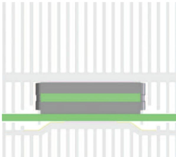
**Figure 6:** A thermal management cell-based design supports power densities in excess of 200 W/in<sup>2</sup> and power outputs to 1.8 kW/cell. The design readily scales for larger systems of multiple cells
