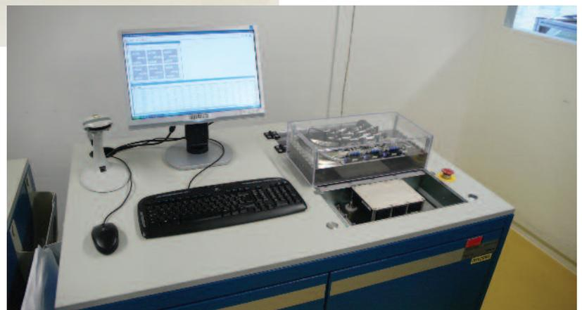
**Figure 2: Baseplate flatness test system**
