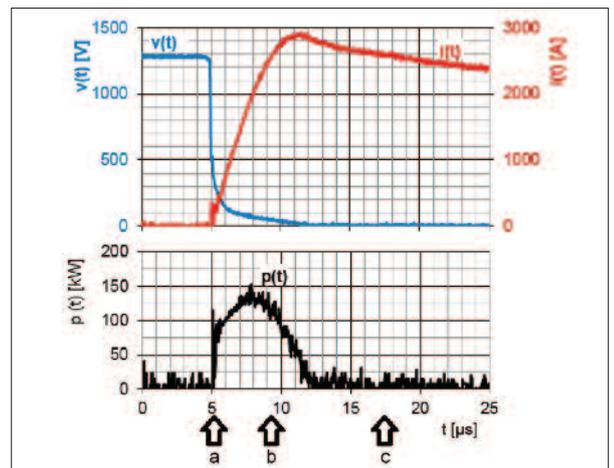
Figure 5 shows the waveforms during thyristor turn-on (600 A/μs) and calculated power loss (arrows below relate to Figure 4),  $T_j = T_{jmax}$ .
