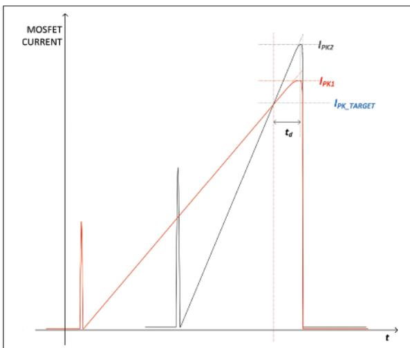
LEFT Figure 3: MOSFET current at different converter input voltage
