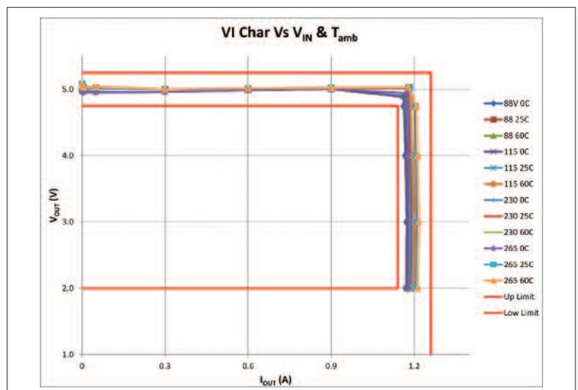
RIGHT Figure 4: Converter voltage / current output curves
