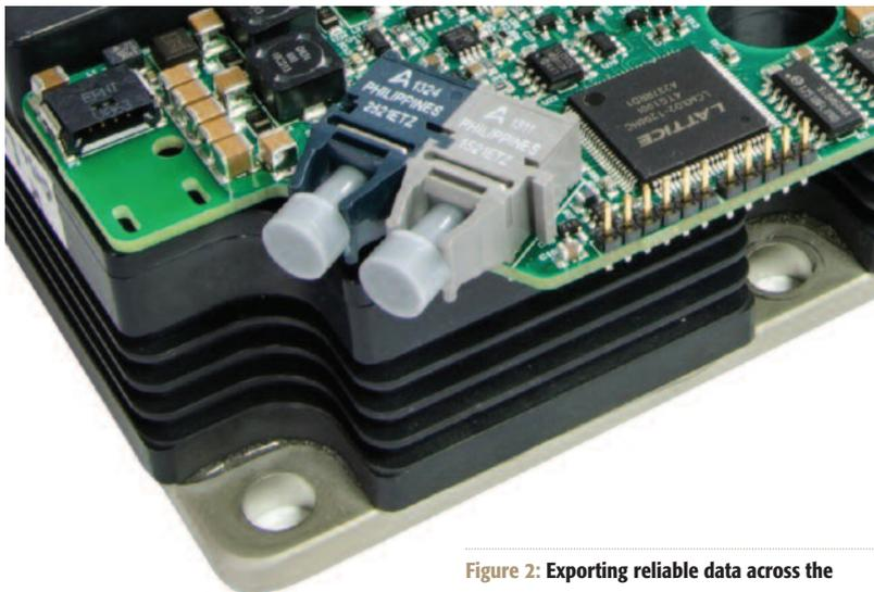
**Figure 2: Exporting reliable data across the isolation barrier**
