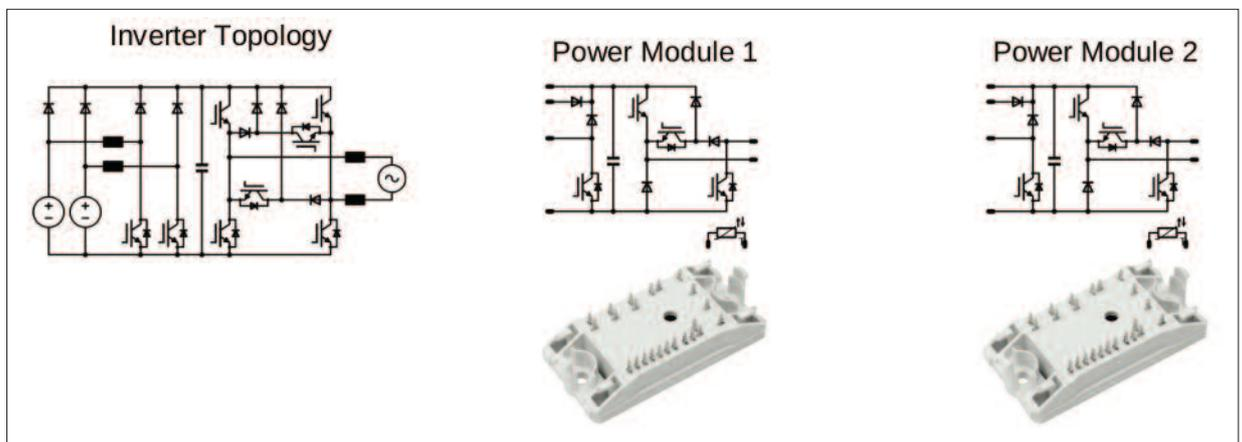
Figure 6: 2x Boost + Halfwave Inverter
