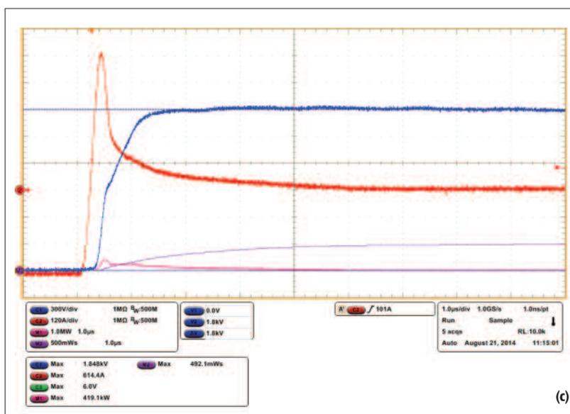
Figure 6: Switching waveforms of FF450R33TE3 for turn-on (a), turn-off (b) and recovery (c) at nominal conditions 1800 V / 125°C
