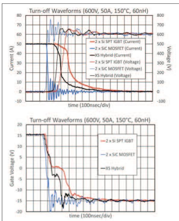
Figure 4: Turn-off switching waveforms comparing the XS hybrid to 2 x Si SPT IGBTs and 2 x SiC MOSFETs at 50 A, 600 V, 150°C
