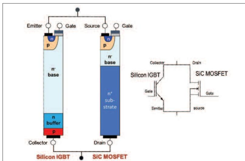
Figure 1: Si IGBT and SiC MOSFET structures for the hybrid Cross Switch
