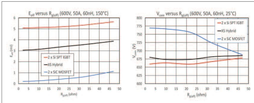
**Figure 5:**  $E_{off}$  at 150°C (left) and  $V_{cem}$  at 25°C as a function of  $R_{g(off)}$  comparing the XS hybrid to 2 x Si SPT IGBTs and 2 x SiC MOSFETs at 50 A/600 V
