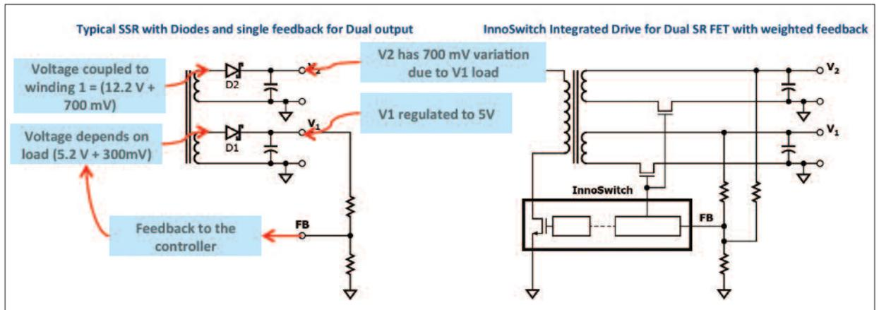
Figure 5: InnoSwitch-EP uses a synchronous rectification MOSFET which is relatively insensitive to changes in load current, reducing cross regulation effects on the other outputs
