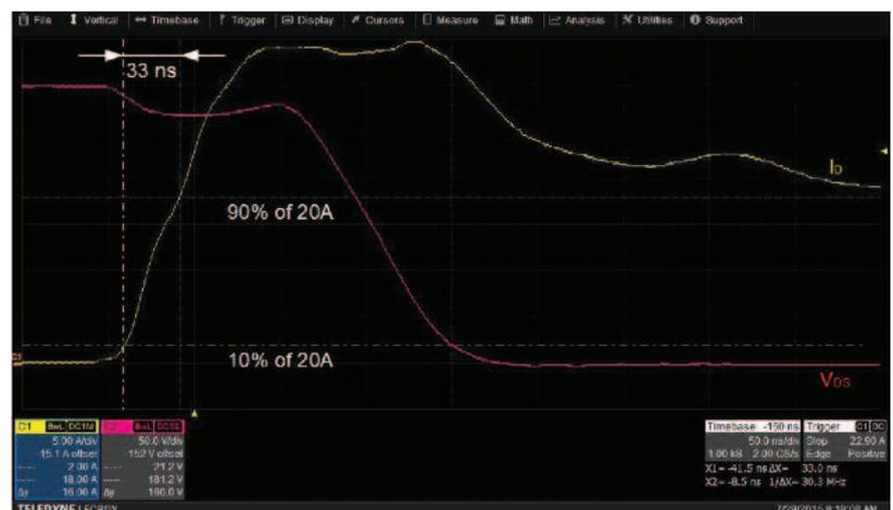
Figure 6: Turn-on behavior of a SiC device (C3M0065090D)
