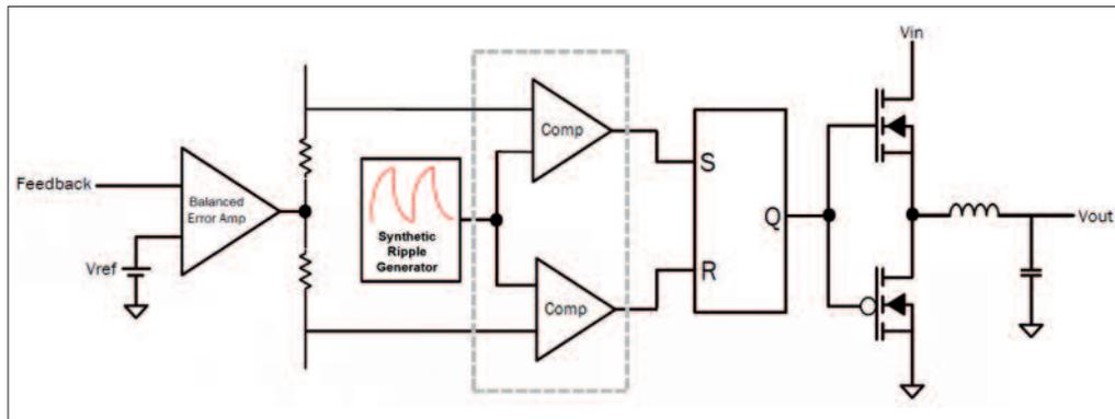
Figure 2: Block diagram of the ISL68200 control loop with synthetic ripple generator
