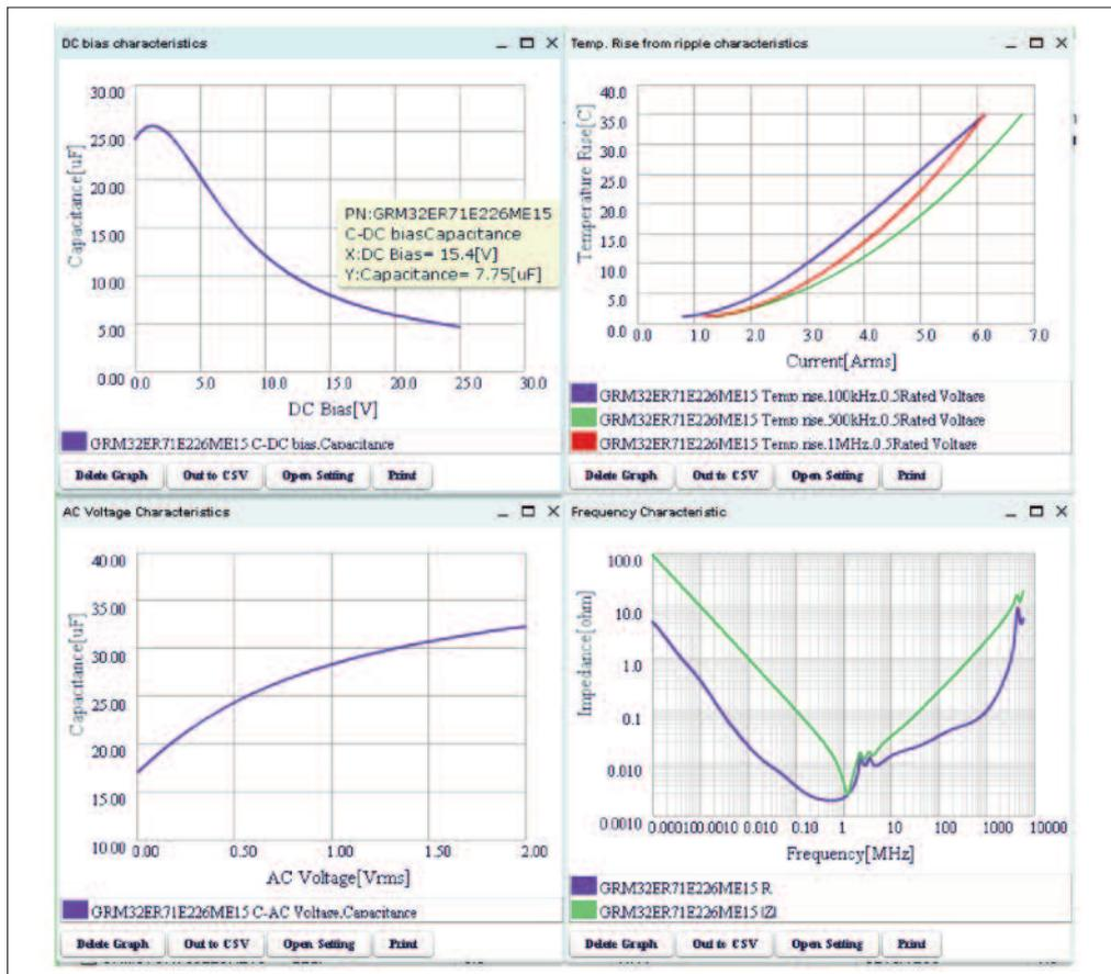
**Figure 1: The SimSurfing simulator shows the behavior of ceramic capacitors and inductors under varying conditions. This plot shows the characteristics of a 22  $\mu\text{F}$  / 25 V capacitor**
