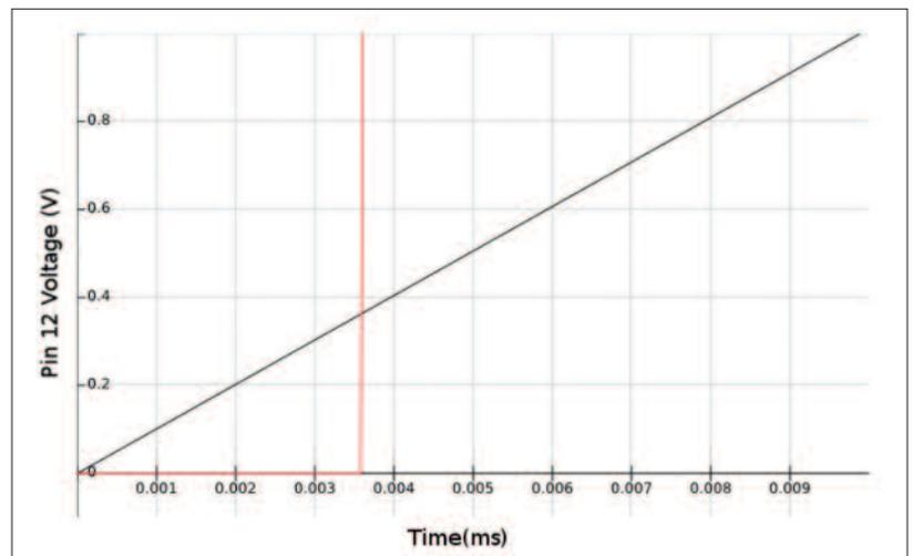
**Figure 2: The first few microseconds of a 230 V/50 Hz mains waveform**
