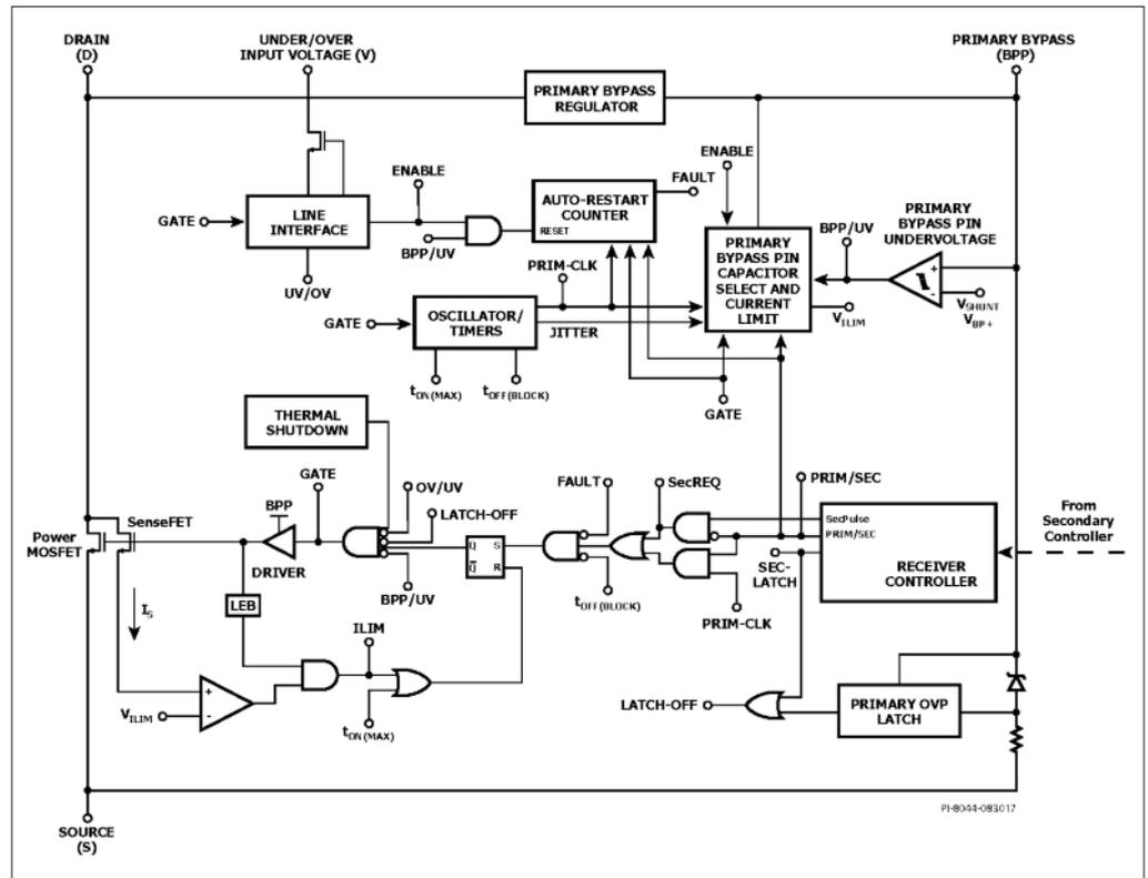
diode / SR FET short protection circuit and a 650 V / 725 V power MOSFET.
