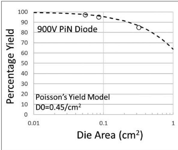
**Figure 1: Percentage yield vs. die area for 900 V PiN diodes (yield is modeled using Poisson's model, assuming defect density of 0.45/cm<sup>2</sup>)**
