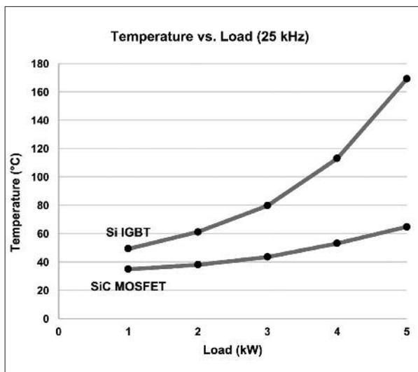
LEFT Figure 6: Switch losses vs. load of simulated converter, showing Si IGBT in red and SiC MOSFET in gray (Note - bench top testing of Si IGBT based converter at 200 kHz is not possible)
