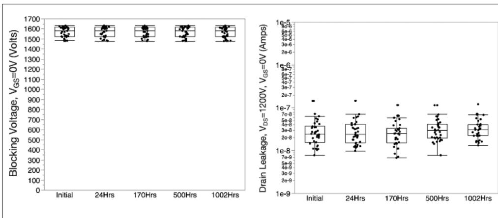
**Figure 2: Results of high temperature reverse bias testing at 175°C (breakdown voltage at  $V_{GS} = 0$  V, leakage current at  $V_{DS} = 960$  V)**
