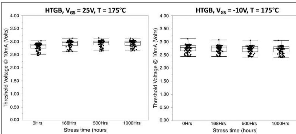
**Figure 3: Results of high temperature gate bias (HTGB) testing at 175°C ( $V_{GS} = -10$ V and at  $V_{GS} = +25$  V)**
