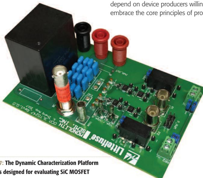
Figure 7: The Dynamic Characterization Platform (DCP) is designed for evaluating SiC MOSFET switching performance
