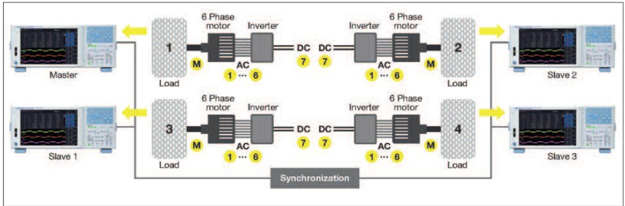
**Figure 4:** By synchronizing four WT5000s with one master unit and three slave units, up to 28 input elements for electrical power measurements and up to 16 motor evaluation functions can be accessed
