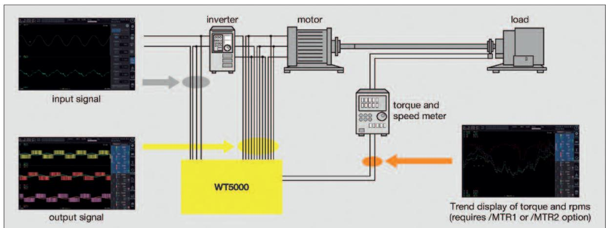
**Figure 3: With multi-channel power measurements, motor evaluation and harmonic comparison capabilities, the WT5000 helps engineers in motor and drive development**
