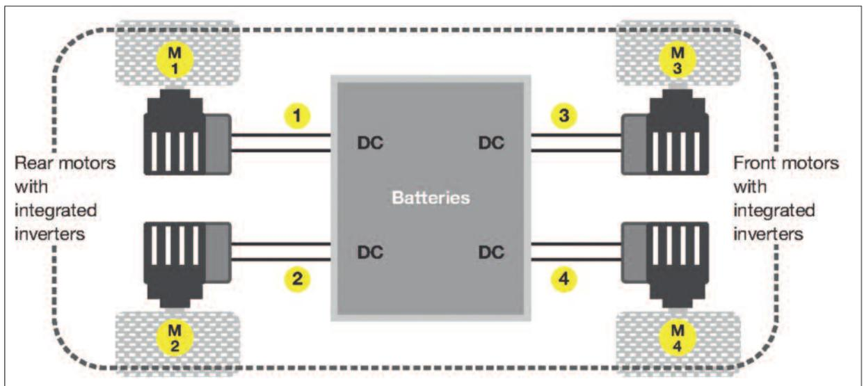
**Figure 5:** Modern drive systems with integrated inverters do not allow access to the AC signals. Here one of the main measurement tasks is to measure the overall drive train efficiency from DC to mechanical power. The example shows 4 DC measurements (1 to 4) with the corresponding 4 mechanical power measurements (M1 to M4)
