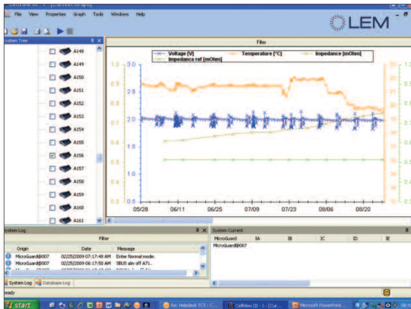
Figure 3: Cell impedance predicts failure
