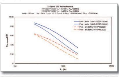
Figure 3: Output power versus switching frequency for a 3-level inverter
