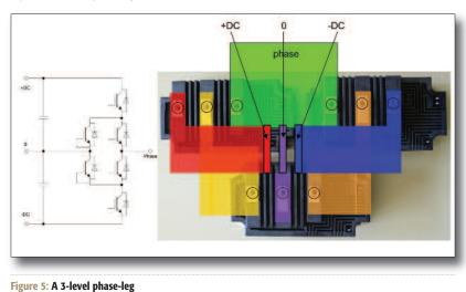
function the integrated free-wheeling diode of the HiPakO Module with shorted gate-emitter can be utilised. This way there is only one kind of module necessary for the 3-level phase leg.
