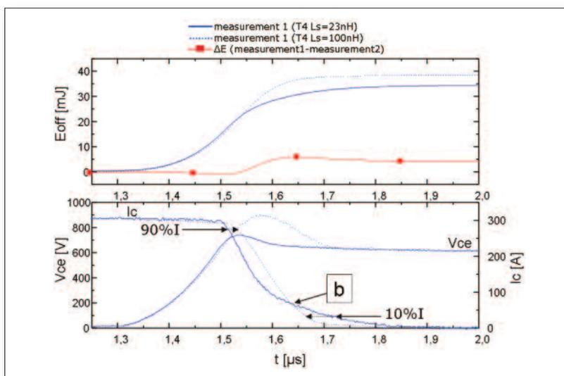
**Figure 3:** Turn-off behavior of a Low Power IGBT; the diagram on the top shows the losses versus the time for two inductances (solid:  $L=23\text{nH}$ , dotted:  $L=100\text{nH}$ ); the bottom diagram shows the voltage and the current curves
