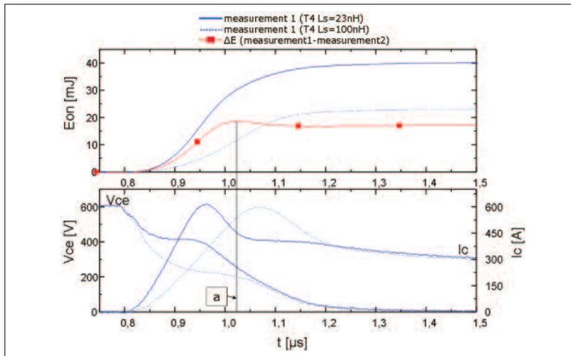
**Figure 2:** Turn-on behavior of a T4; the diagram on the top shows the losses versus the time for two inductances,  $L=23\text{nH}$  and  $L=100\text{nH}$ ; the bottom diagram shows the voltage and the current curves
