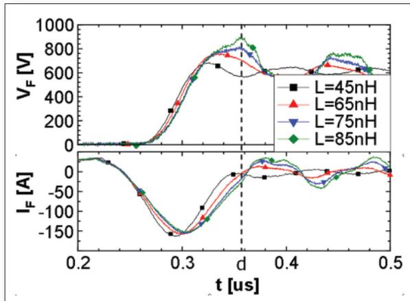
**Figure 7: Diode recovery at room temperature and 1/10  $I_{nominal}$ ; curves for different stray inductances**
