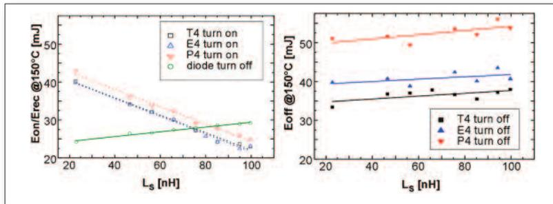
**Figure 5: Switching losses as function of the stray inductance  $L_s$ , the turn-on losses of the IGBT (left) will be reduced by increasing the inductance and the turn-off losses of the IGBT, right, and the freewheeling diode rise with the inductance**
