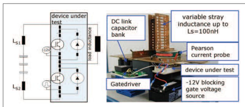
Figure 1: Test set-up, for recovery measurement of the free wheeling diode the high side IGBT was switched and the load inductance was changed to be parallel to the low side diode
