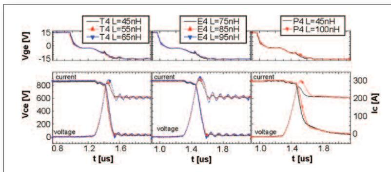
**Figure 6: Switching curves as function of the stray inductance  $L_s$  of three IGBT versions; T4 (left), E4 (middle), P4 (right); the diagrams on the top show the gate voltage; the diagrams on the bottom show the current and voltage curves**
