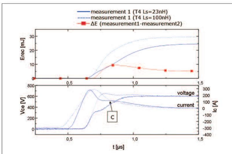
**Figure 4:** Recovery of the diode: the diagram on the top shows the losses versus the time for two inductances (solid:  $L=23\text{nH}$ , dotted:  $L=100\text{nH}$ ); the bottom diagram shows the voltage and the current curves
