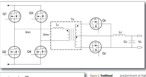
Figure 2: Phase-Shifted Full-Bridge Converter
