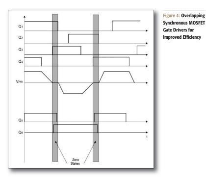
synchronous MOSFET's PWM gate drive, high secondary currents flow through MOSFET channel. In this instance, there will be only  $R_{ds(ON)}$  losses, which are much less than the losses incurred by the MOSFET body diodes in the dead time. For a system with a telecom input (36 to 76 VDC), the DC/DC converter's efficiency improves anywhere from 3-4% by overlapping the synchronous MOSFET gate drive.
