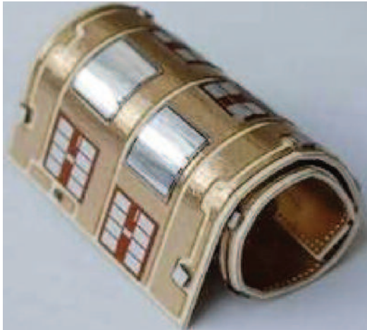
Figure 3: DBC substrate after mechanical stress test
