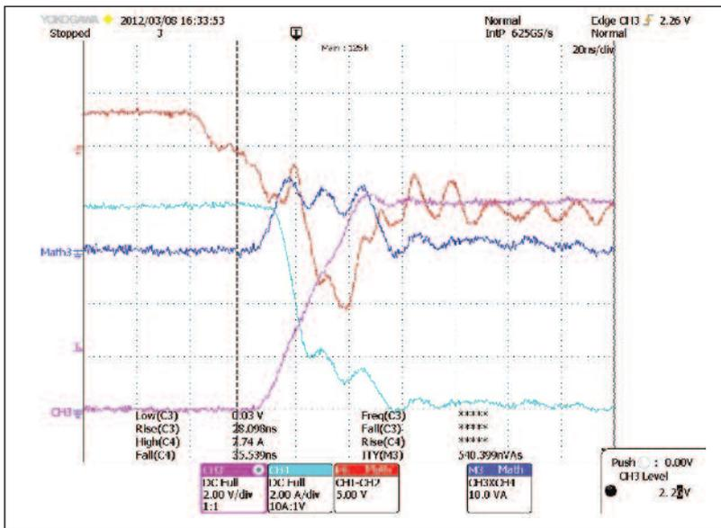
**Figure 9: Turn-off waveform in BCM at  $V_{out} = 800 V$  ( $E_{off} = 54 \mu J$ , M1 red... $V_{ce}$ , M3 dark blue... $E_{on}/E_{off}$ )**
