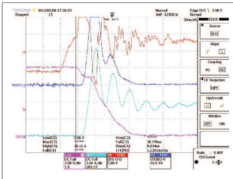
**ABOVE Figure 6:  $E_{on}$  measurement in CCM** ( $E_{on} = 113 \mu J$ , Ch3 magenta... $V_{ce}$ , Ch4 blue... $I_c$ )
