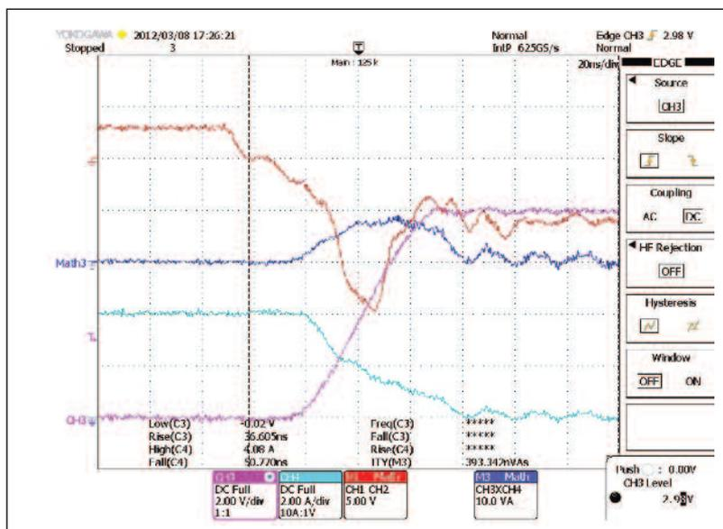
**LEFT Figure 7:  $E_{off}$  measurement in CCM** ( $E_{off} = 51 \mu J$ , M1 red... $V_{ce}$ , M3 dark blue... $E_{on}/E_{off}$ )
