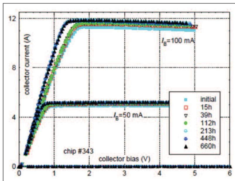
Figure 1: Gain (hFE) and  $V_{CE(SAT)}$  before and after 660 hour DC stress test (open collector,  $I_{Bc}=0.25$  A)
