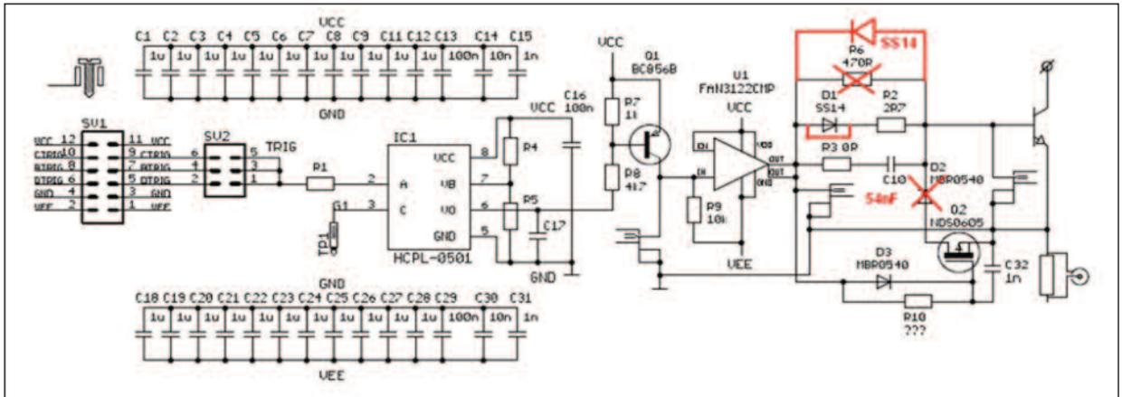
Figure 2: Base drive circuit for SiC BJT
