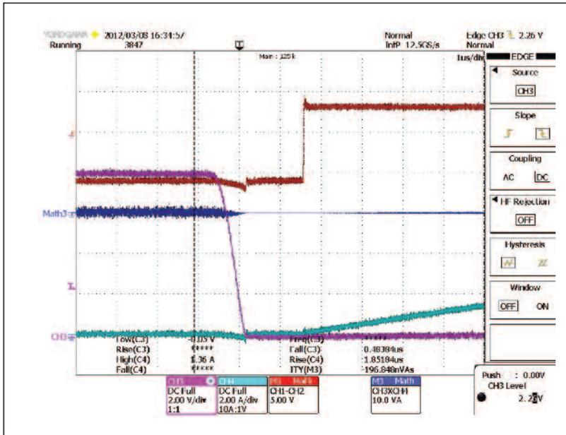
**LEFT Figure 8: Smooth turn-on of the SiC BJT in ZVS ( $E_{on} = 0 \mu J$ ,  $V_{out} = 800 V$ , Ch3 magenta... $V_{ce}$ , Ch4 blue...I)**
