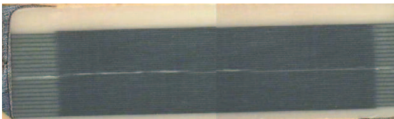
Figure 7: Piezo stress crack failure
